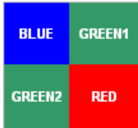
Figure 4. Color Filter Arrangement on the Pixels
